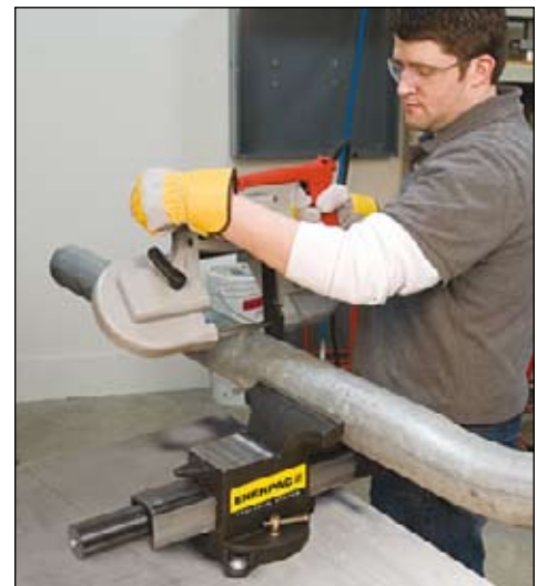
Enerpac BV-5 Hydraulic Bench Vise with hands-free PA-133 Foot Pump makes work with a large heavy piece into a one person job.
