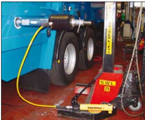
◀ An RACH-306 powered by a P-392 hand pump used to extract corroded carriage pins of refuse collection vehicles.
