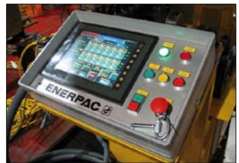
▲ PLC-controller station for ESS-Series synchronous lifting system.
