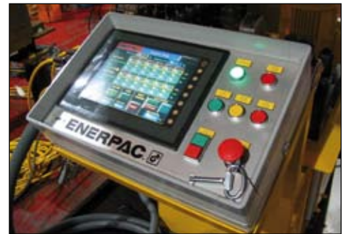
▲ PLC-controller station for ESS-Series synchronous lifting system.
